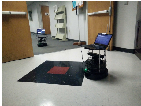
Figure 4.1: The robots, TurtleBots 2 equipped with a Wi-Fi dongle, deployed in an environment to build its communication map.
